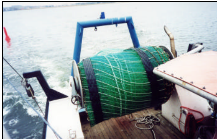
Figure 5: Conventional seagoing vessel with equipment for lowering and pulling in the special net (prototype)
