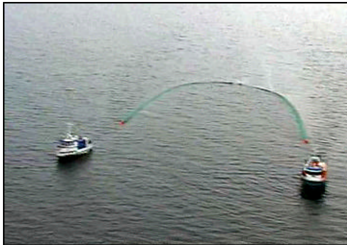
Figure 4: Field test with a prototype of a surface controlled net
