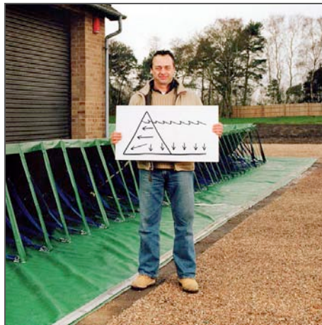
Figure 15. Mobile flap system made of flexible plastic material (Rapidam, 2010)
