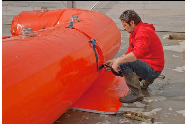
Figure 6: Corner element of the prototype Optimal in a laboratory test of the research project HWS-MOBILE (photo: B. Koppe)
