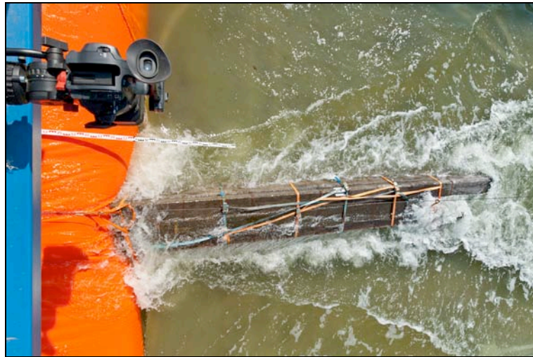
Figure 10: Flotsam impact test at water-filled tube prototype Optimal within the research project HWS-MOBILE (photo: B. Koppe)
