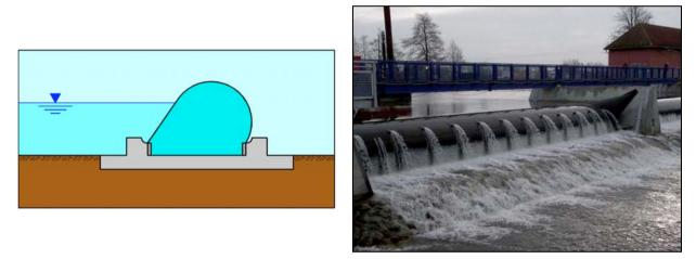
Figure 2: Construction principle of a permanent installed tube system (left) and an example of a water-filled weir in Marklendorf at the river Aller, Germany<sup>7</sup> (right)
