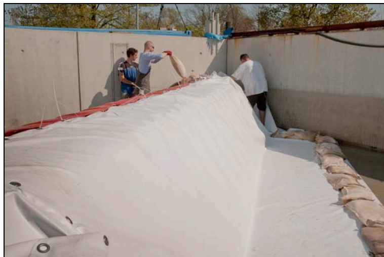
Figure 9: Laboratory test of the prototype Daedler with a waterside placed plastic sheet on an impermeable ground within the research project HWS-MOBILE (photo: B. Koppe)
