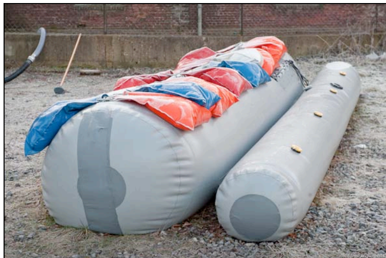
Figure 11: Water-filled, sandbag loaded prototype Optimal after a several months lasting freezing period in January 2011, research project HWS-Mobile (photo: B. Koppe)
