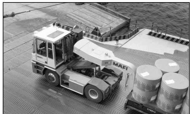
Figure 2 Tractor equipped with gooseneck and roll-trailer [6]
