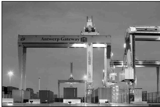
Figure 7 Rail mounted gantry crane in the Port of Antwerp [9]
