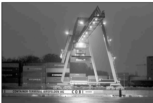
Figure 8 Rail mounted wide span gantry crane at the Port of Birsfelden, Switzerland [9]
