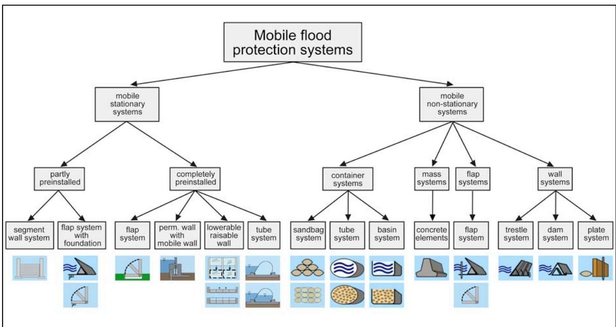
Figure 1: Classification of mobile flood protection systems<sup>6</sup>
